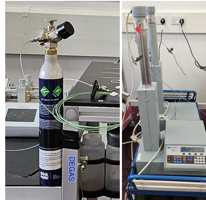
Figure. ISCO pump machine and CO 2 gas with its regulator.
