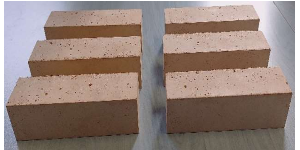
Mortars were cast into prismatic molds ( 40 \times 40 \times 160 mm)
