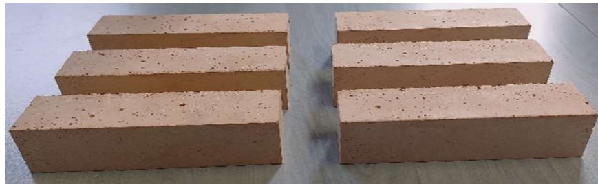
Mortars were cast into prismatic molds (40 × 40 × 160 mm)
